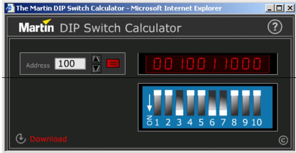
One way to find DIP-switch settings is to use a DIP-switch calculator. You enter the address in the calculator and it displays the proper DIP setting. Just set the switch as shown in the display.
